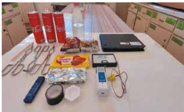
Figure 2: Equipment and materials for the exercise Energy from Food (Phywe CobraSmart Thermocouple sensor was used to measure temperature changes)
